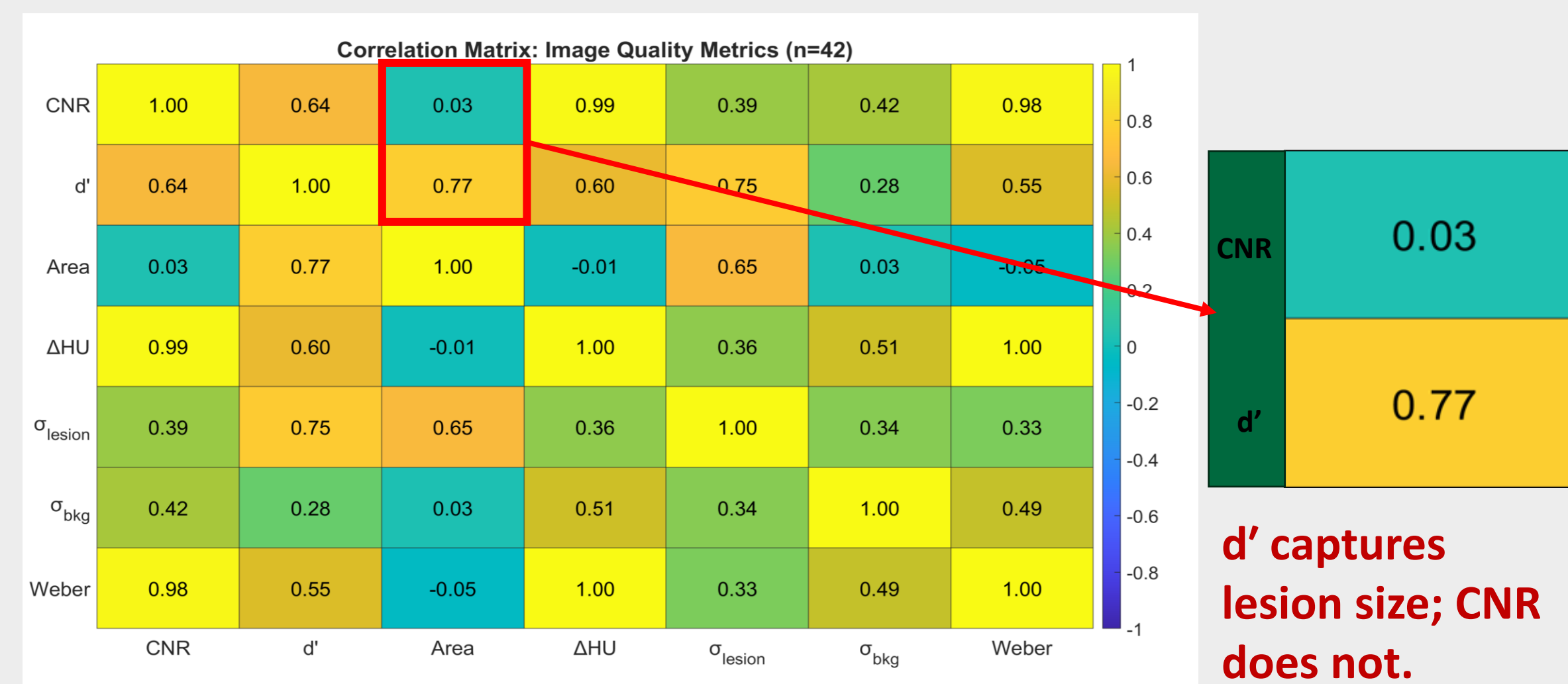
Figure 2. Pearson correlation heatmap of image quality metrics ( n=42 ). CNR correlates near-perfectly with lesion contrast ( \Delta HU : r=0.99 ) and Weber contrast ( r=0.98 ) but not with lesion area ( r=0.03 ). Detectability index ( d' ) correlates with both area ( r=0.77 ) and contrast ( r=0.60 ), capturing geometric factors CNR misses. Color scale: -1 (blue) to +1 (yellow).
