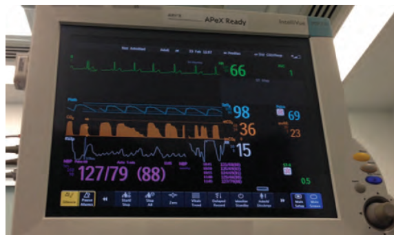
Figure 4. Photograph of a patient monitor screen, as viewed during sedation. During moderate sedation, the patient's blood pressure (purple numbers), heart rate (green rhythmic pattern), oxygen saturation (blue waveform), end tidal carbon dioxide partial pressure (orange waveform), and respiration rate (white waveform) are monitored.
